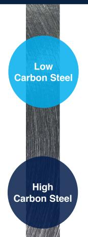
The hardness or temper of cold rolled mild steel strip is determined by its analysis, the amount of cold rolling or by a final annealing process. These are selected to achieve the optimum mechanical properties for the forming operation whether it be deep drawing, forming or flat blanking. "Skin passed" is a very light rolling reduction after the annealing process to prevent the formation of deformation bands called stretcher strains, which can ruin surface appearance of the formed article.
